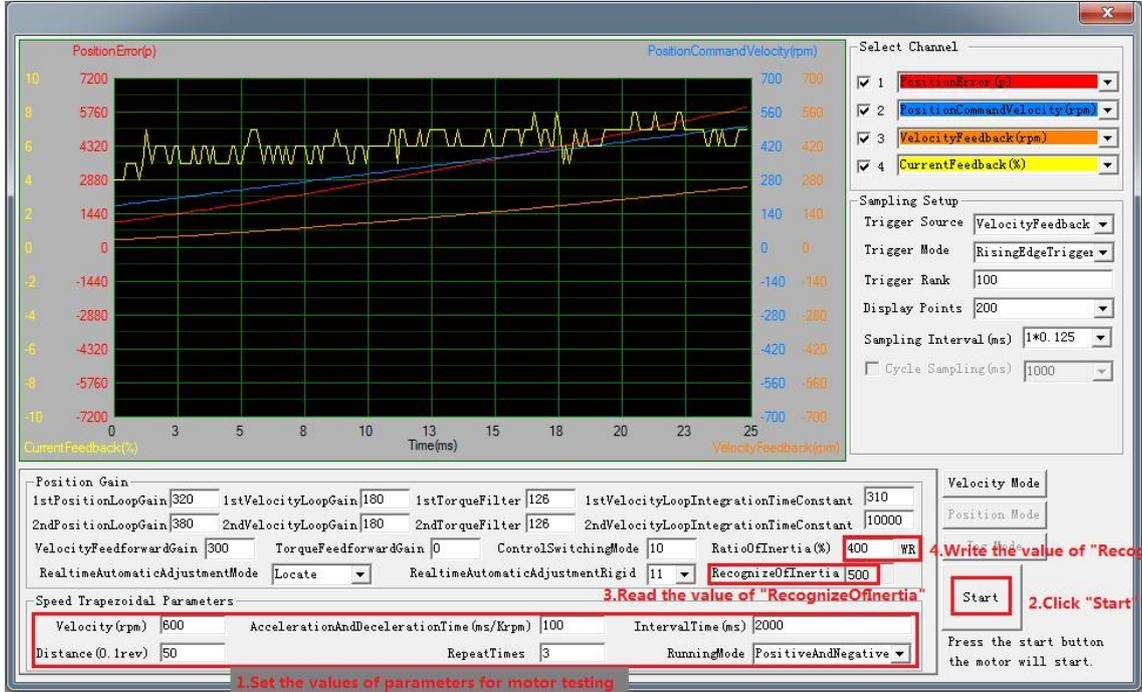
The screenshot shows the software interface with a graph and parameter settings. The graph displays PositionError(p) on the left y-axis (ranging from -10 to 10) and PositionCommandVelocity(rpm) on the right y-axis (ranging from -700 to 700) against Time(ms) on the x-axis (ranging from 0 to 25). Below the graph, various parameters are set, including Position Gain, Velocity Mode, and Speed Trapezoidal Parameters. Red boxes and annotations highlight specific steps:
