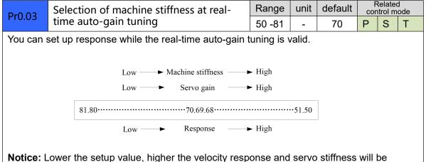
**Notice:** Lower the setup value, higher the velocity response and servo stiffness will be obtained. However, when decreasing the value, check the resulting operation to avoid oscillation or vibration.
