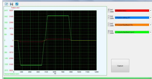
As keep decreasing the value pf Pr0.03, the position loop gain Kp become bigger and bigger, the integration time constant Vi become smaller and smaller, the position error become close to zero. Pr0.03=61
