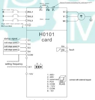
wiring diagram of carving maching inverter
