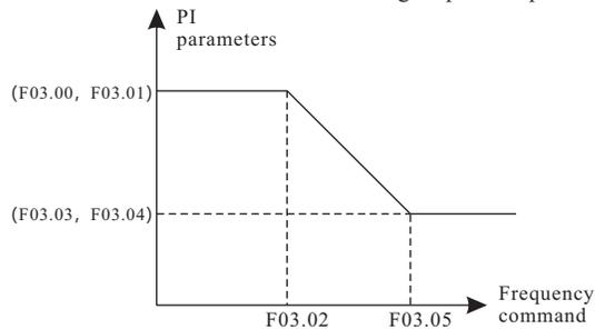
Figure 6-5 Relationship between running frequencies and PI parameters
