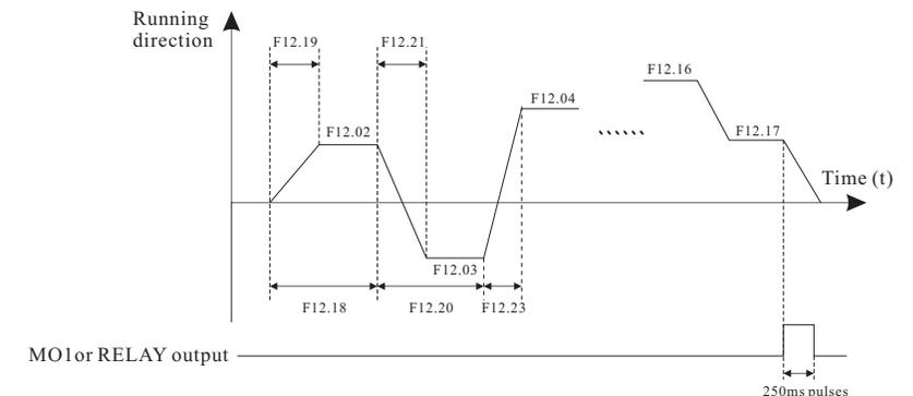
Figure 6-34 Simple PLC when used as frequency source
