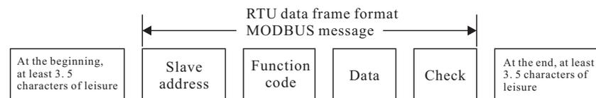
The standard structure of RTU frame:
