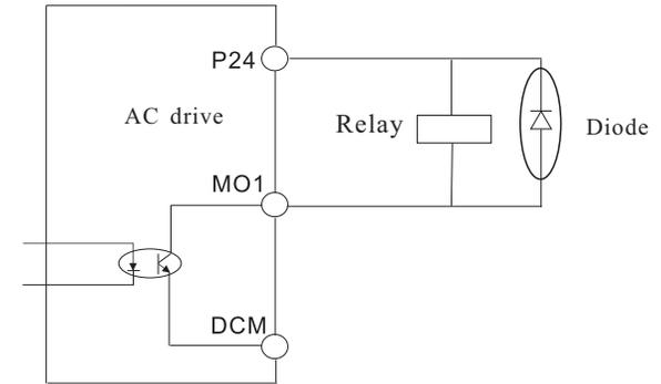
Figure 3-7 Wiring diagram of digital output terminal
