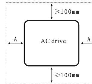
Explanation: When power of AC drive ≤22kW it means taking no account of size A is permissible. When the power >22kW, A shall be larger than 50mm.
