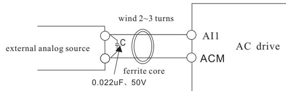
Figure 3-6 Analog input terminal with filter devices
