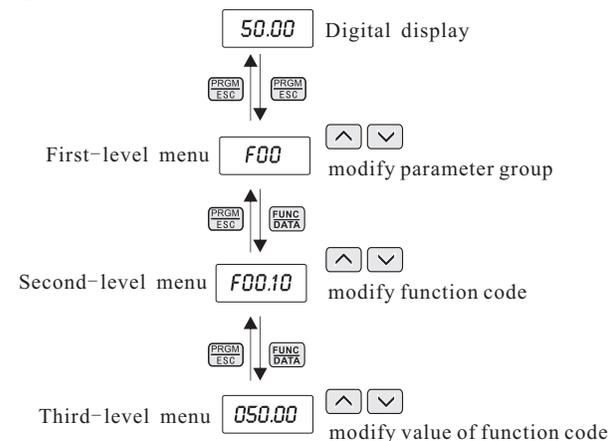
Figure 4-2 Operation flow chart of three-level menu
