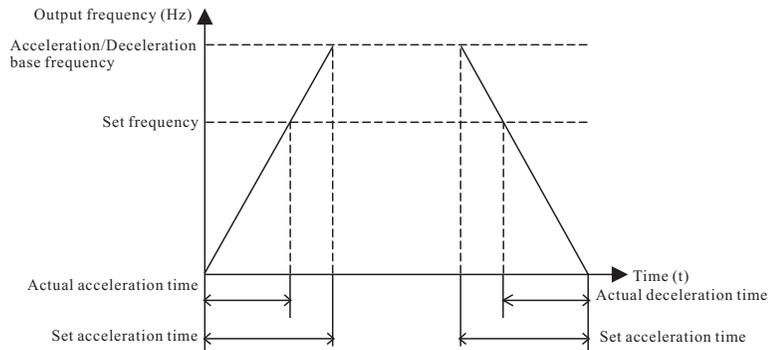
Figure 6-1 Acceleration/Deceleration time
