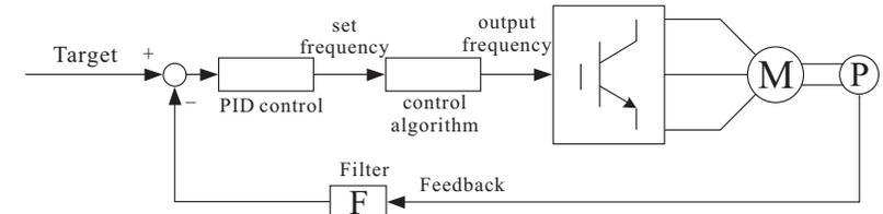
Figure 6-28 Principle block diagram of PID control
