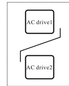
Explanation: When AC drive is installed upside and underside, please install thermal insulation guide plate as picture shows.
