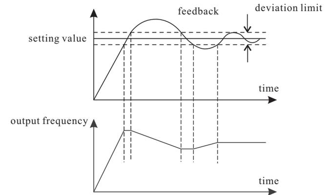
Figure 6-29 relation between deviation limit and output frequency
