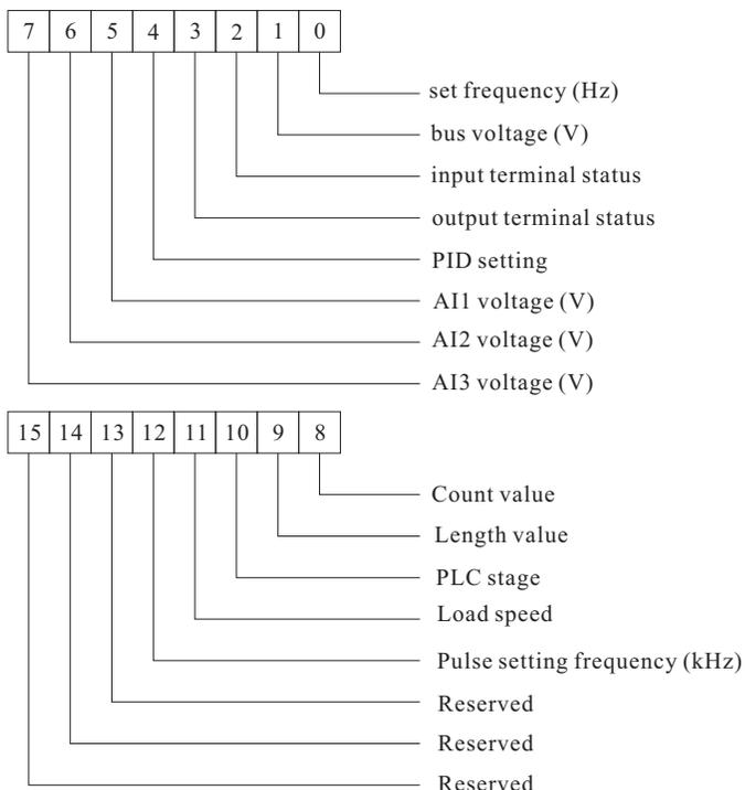
If a parameter needs to be displayed during the running, set the corresponding bit to 1, and set F07.05 to the hexadecimal equivalent of this binary number.
