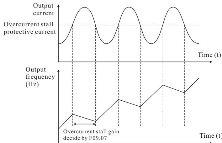
Figure 6-27 Diagram of the overcurrent stall protection function
