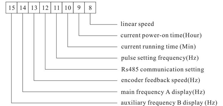
If a parameter needs to be displayed during the running, set the corresponding bit to 1, and set F07.04 to the hexadecimal equivalent of this binary number.
