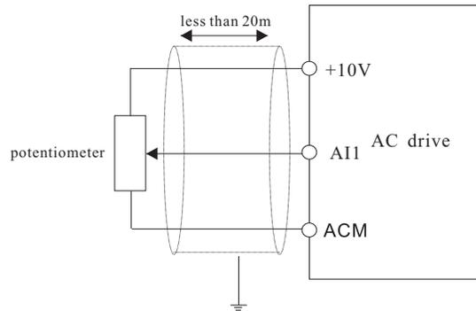
Figure 3-5 Schematic diagram of analog input terminal wiring
