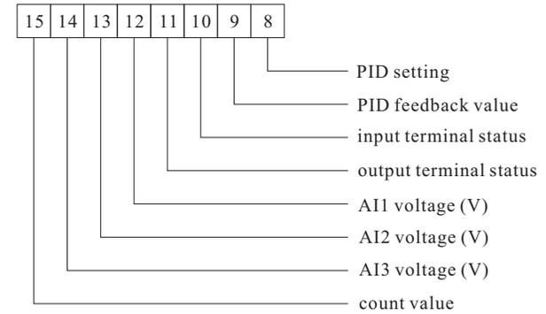
If a parameter needs to be displayed during the running, set the corresponding bit to 1, and set F07.03 to the hexadecimal equivalent of this binary number.
