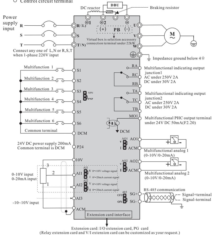
Notes: The general type AC drives  $\leq 22\text{kW}$  have built-in brake unit, brake resistance (+) and PB terminal; (+) and (-) terminals are the plus or minus terminals of inverter's DC bus.
