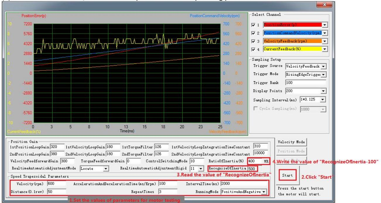
The screenshot shows the motor control software interface. The top part features a graph with four data series: PositionError(p) (red), PositionCommandVelocity(rpm) (blue), VelocityFeedback(rpm) (orange), and CurrentFeedback(%) (yellow). The x-axis represents Time(ms) from 0 to 25. The y-axes represent PositionError(p) from -10 to 10, PositionCommandVelocity(rpm) from -700 to 700, VelocityFeedback(rpm) from -700 to 700, and CurrentFeedback(%) from -10 to 10.
